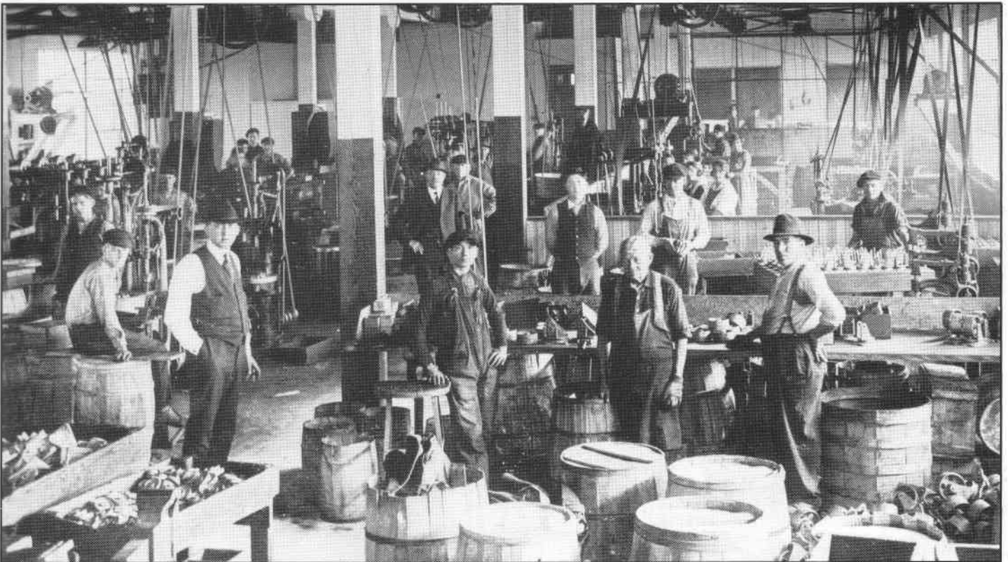
"Team Picture Day" 1920 style. These photos give a view of how we manufactured Casters in the early years. Machines were powered by the overhead line shafts which turned the belts. Most casters in that era were shipped in wooden barrels.
